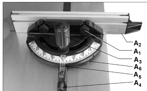
Figure 7-2: Miter Gauge Adjustments
